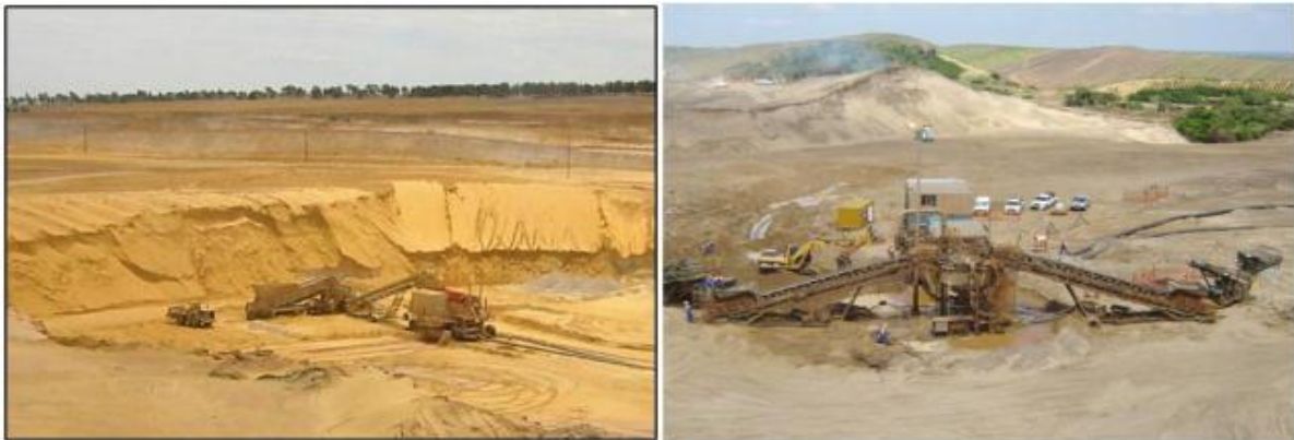
Plate 2.1: Typical loader and hopper dry mining operation
