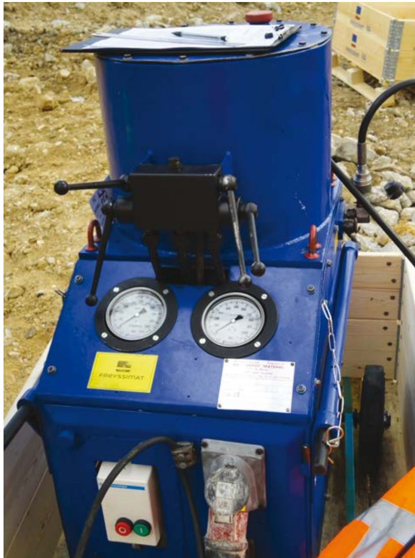
Picture I.3: Hydraulic pump to power the stressing jack (© Freyssinet)
