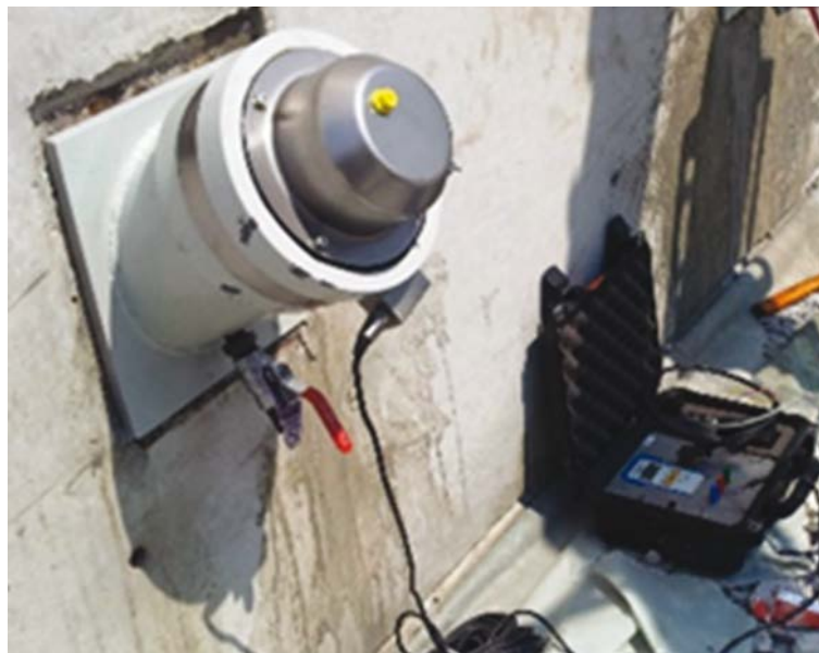
Picture 8.8: Anchor head instrumented with a type P protection (© Soletanche Bachy)
