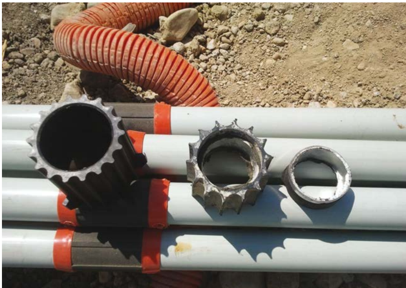
Picture 4.4: spacers set on tubes à manchettes (© Freyssinet)
