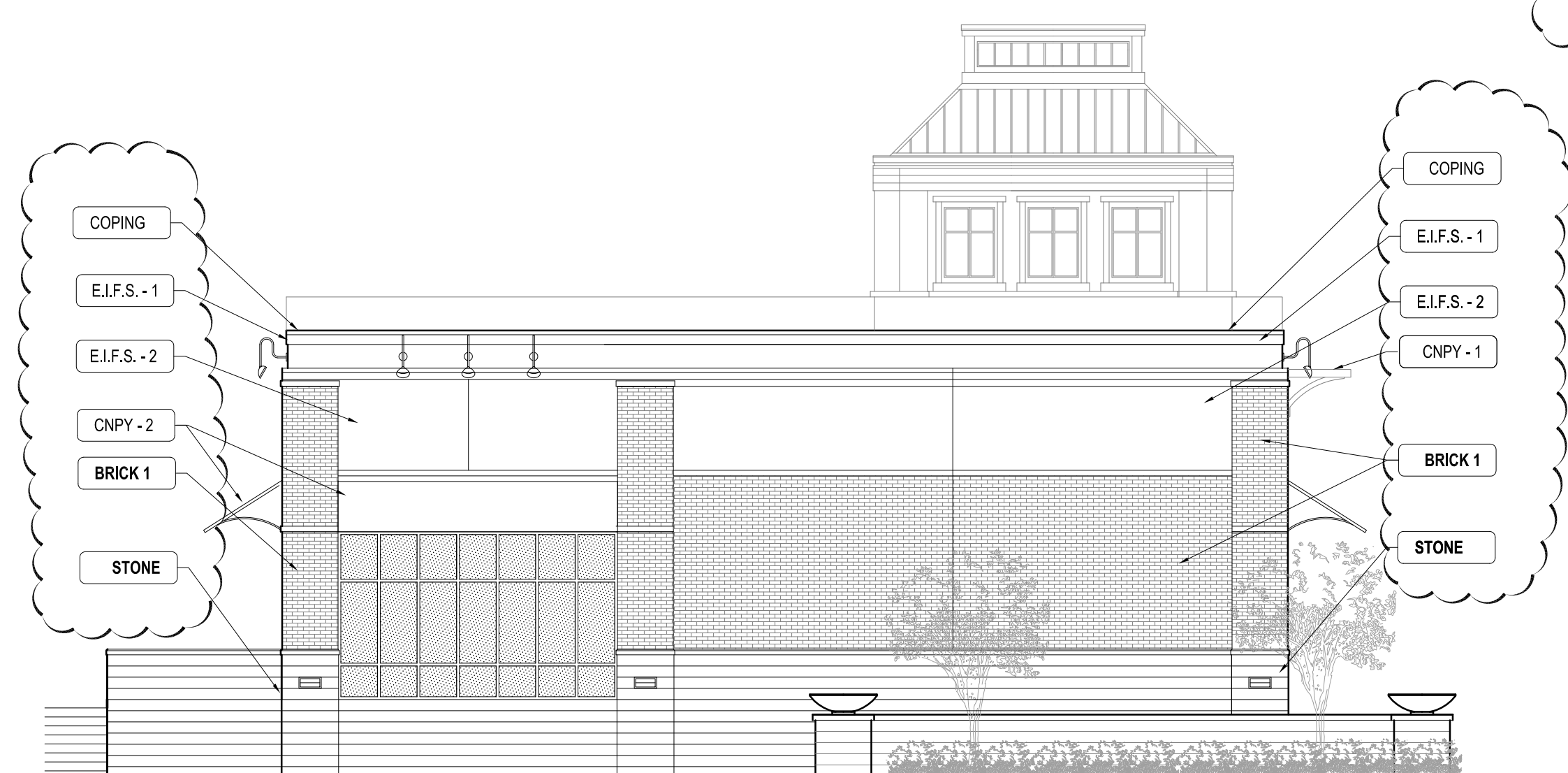
5 EAST ELEVATION AT ENTRY DRIVE SCALE: 1/8" = 1'-0"
