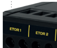
5 On-Off pulse inputs
