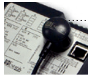
Local communication via optical head
