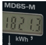
Display of energy index on a LCD screen
