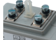
Split output terminals enabling risk-free short-circuiting of the secondary current (M4 or cage for 4 mm 2 wire)
