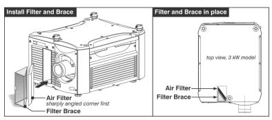
3. Replace the filter door and secure it with (1) screw.
