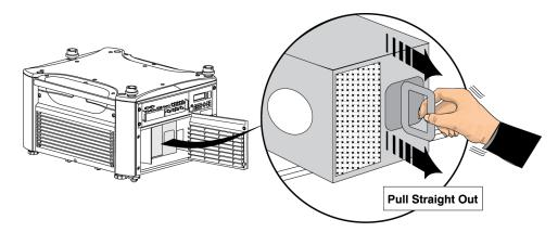
• Grasp the handle on the lamp module and pull the module straight out of the lamp compartment.
