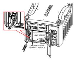
• Pull the lamp module handle outward to remove the lamp.
