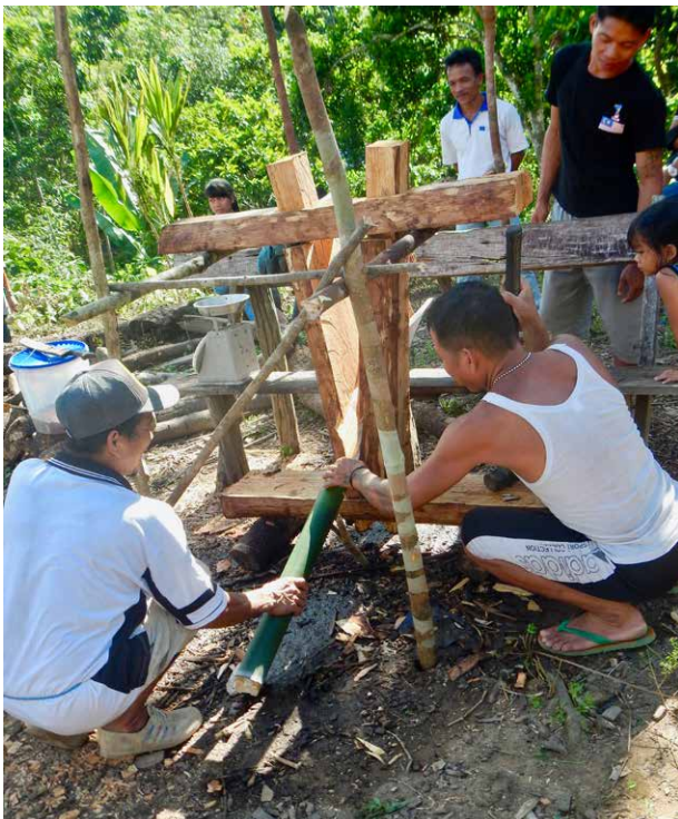
Figure 39. A traditional wooden press to extract the tengkawang (illipe nut) oil from the nuts
