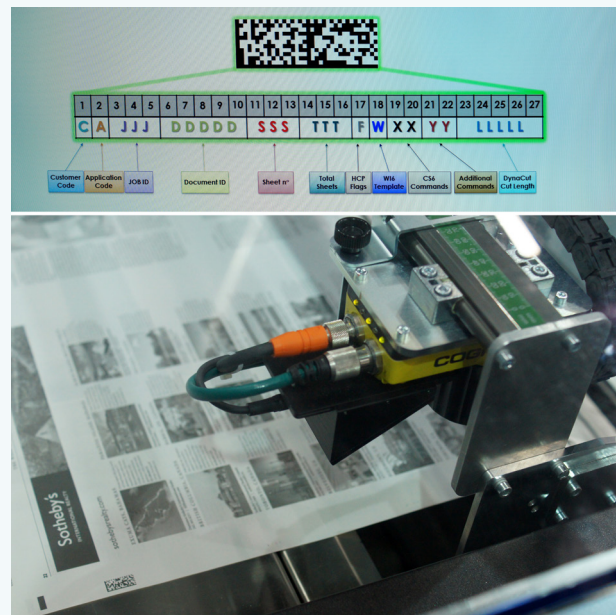
Figure 8: Hunkeler uses inline cameras to capture Data Matrix codes for production monitoring in digital web printing. The mini cameras can also be used to check selected quality parameters. (Photos: Dieter Kleeberg)
