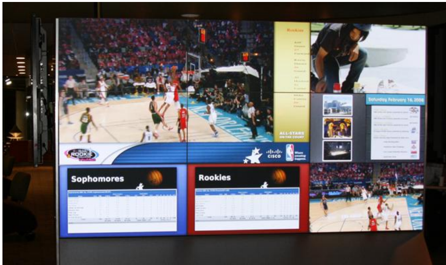
Figure 32. 3x3 Video wall with a 2x2 tile matrix and 5 individual screens
