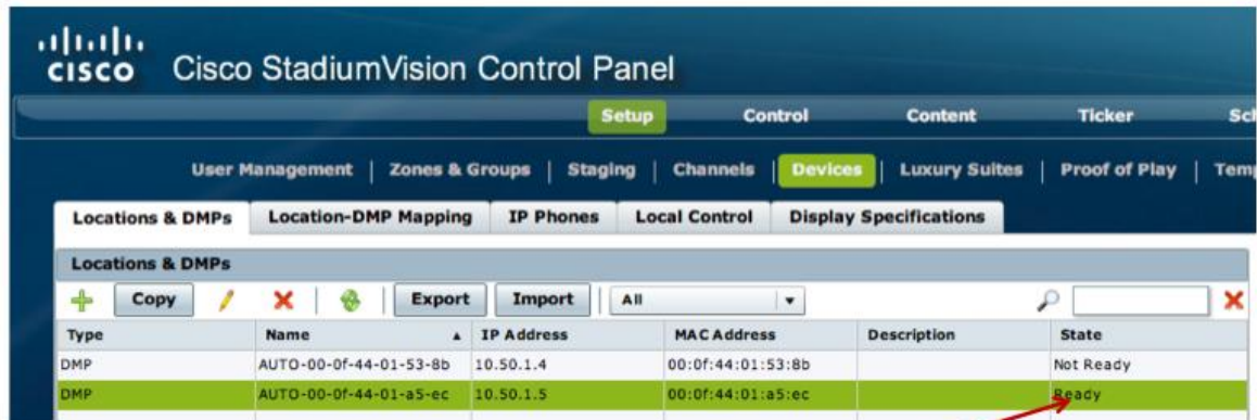
Figure 40. Provisioned DMPs in the Control Panel
