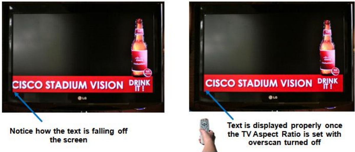
Figure 69. Adjusting the TV's Aspect Ratio
