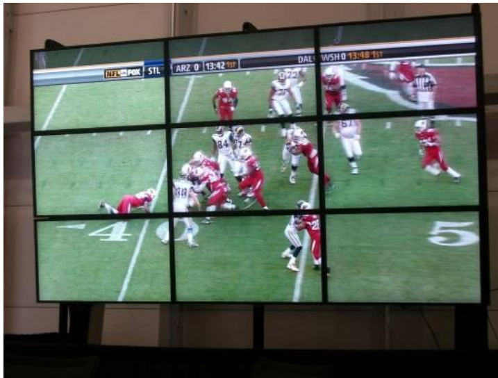
Figure 28. 3X3 Video Wall in Tile Matrix Mode
