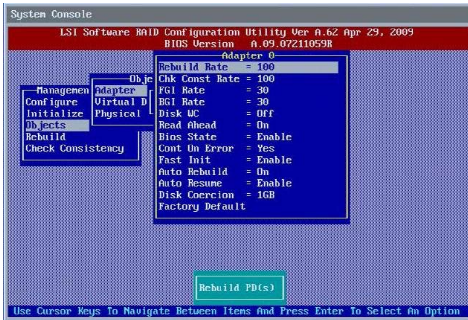
Figure 83 Controller Properties Screen
