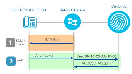
MAB requires a MAC address database | ISE can build this database dynamically with profiling
