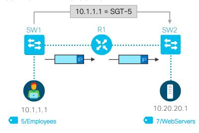
IP-to-SGT data shared over control protocol. No SGT in the data plane. Methods include, IP-to-SGT exchange over:
