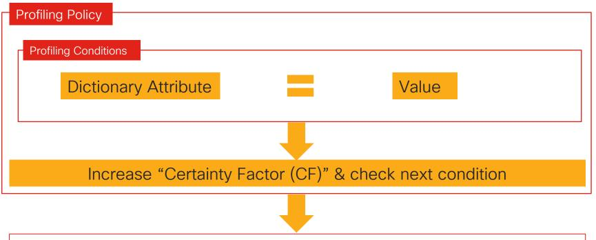
If "CF" > Threshold, Apply Profile & Optionally Assign Endpoint to Group
