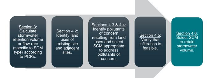
Figure 13. Process for Selecting an SCM
