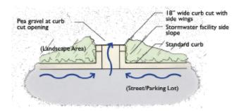
Figure 4-7: Standard curb cut with side wings: plan view (Source: SMCWPPP 2009)
