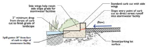
Figure 4-6: Standard curb cut with side wings: cut section view (Source: SMCWPPP 2009)
