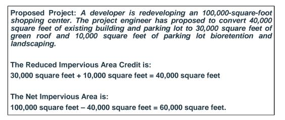
The designer shall use the Performance Requirement Worksheet and SCM Sizing (Appendix A) to determine which PRs apply to the project by inputting project site area information, such as pervious and impervious areas.
