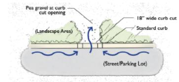
Figure 4-4: Standard curb cut: plan view (Source: SMCWPPP 2009)
