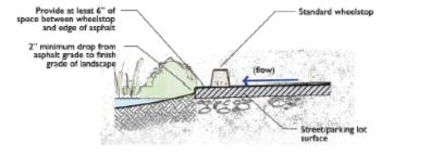
Figure 4-9:Opening between wheelstop curbs: section view (Source: SMCWPPP 2009)
