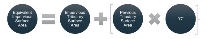
Figure 11. Equivalent Impervious Surface Area Equation
