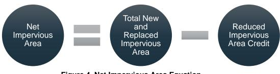
Figure 4. Net Impervious Area Equation
