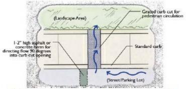
Figure 4-13: Grated curb cut: plan view (Source: SMCWPPP 2009)
