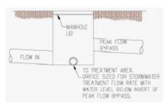
Figure 4-14: Stepped manhole design directs low-flows to treatment measure and diverts high flows to storm drain system. (BKF Engineers)
