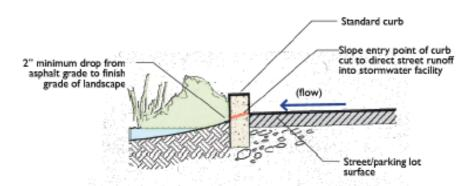
Figure 4-3: Standard curb cut: section view (Source: San Mateo Countywide Water Pollution Prevention Program [SMCWPPP] 2009)
