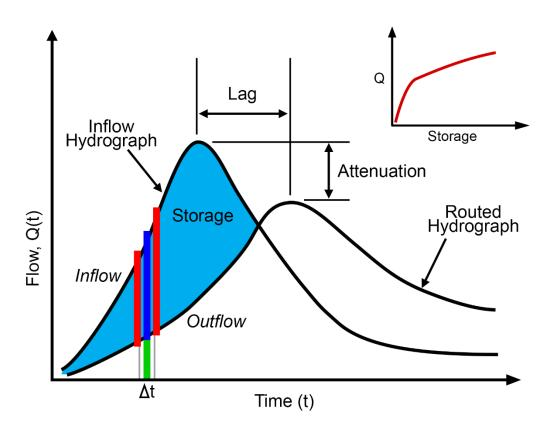
Figure 9. Hydrograph with Flow and Stage Storage
