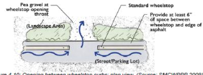
Figure 4-10: Opening between wheelstop curbs: plan view (Source: SMCWPPP 2009)
