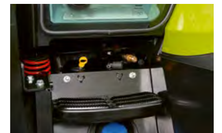
NEW: Compressed air connection on the left side of the access steps.
