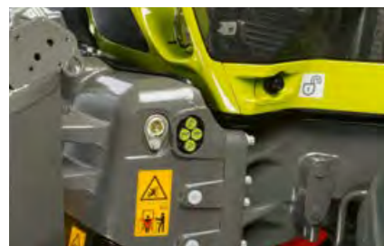
External controls for the front linkage and one spool valve (depends on installed equipment).
