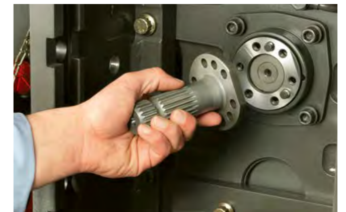
The PTO stub can be changed easily.
