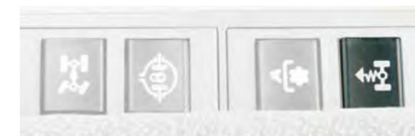
Switch to activate front axle suspension.
