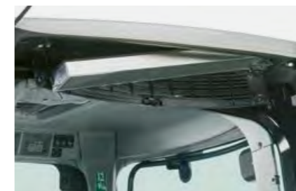
Easy access to the cab air filter on the cab roof.
