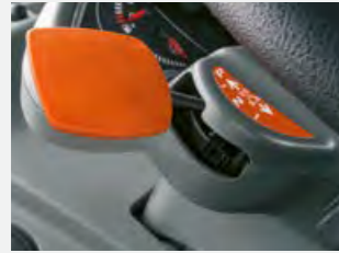
REVERSHIFT clutchless reverser with electronic parking brake available.
