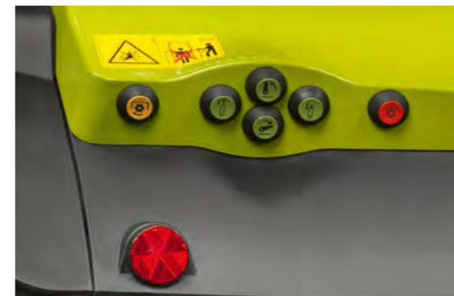
External controls for rear PTO.
