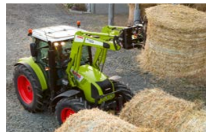
98 l/min maximum hydraulic pump capacity for fast front loader work
