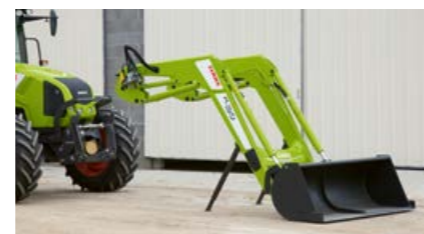
The CLAAS front loader rests safely on the attachment and support legs.
