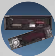
Detachable control panel
