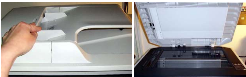
The KX-MB3020's 50-sheet automatic document feeder (left) and platen glass (right).
