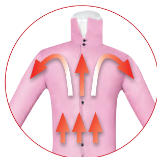
Set the timer to the necessary period – the article of clothing is dried and ironed by the air flow
