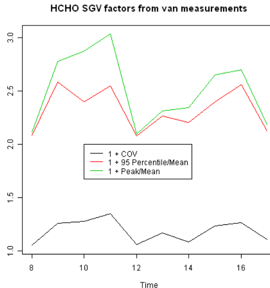
Fig. 4. Three different forms of SGV parameterization derived from mobile van measurements during the July 31 – August 5, 2005 summer campaign
