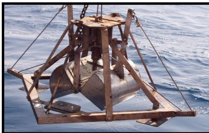
**Fig.2. Smith-McIntyre Grab sampler (Photo courtesy: CMLRE)**
