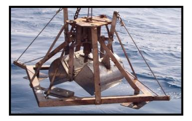
Fig.2. Smith-McIntyre Grab sampler (Photo courtesy: CMLRE)
