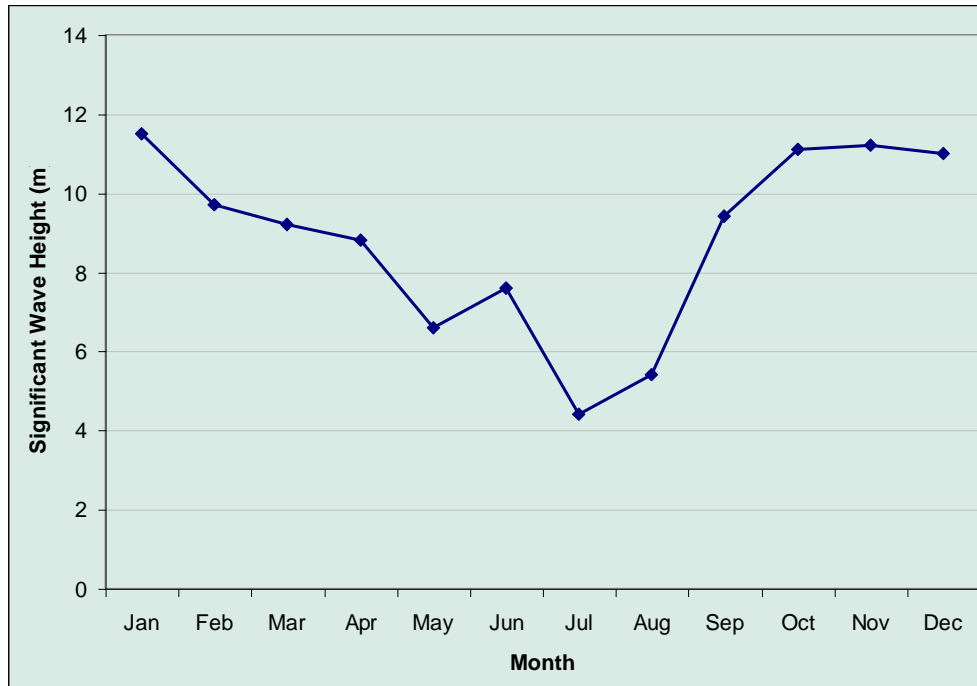
Figure 4-12 Maximum Significant Wave Height for the MSC50 Grid Point (M3013763)
