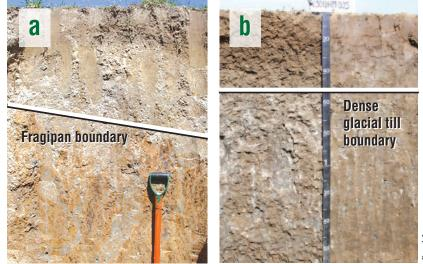
**Figure 1.** Cross-section of restrictive layers in soils formed by a fragipan (a) and dense glacial till (b). Water collects on top of these very slowly permeable layers in winter and spring resulting in saturated soil conditions and a seasonally high "perched" water table. Notice that the layers' upper boundaries are not always parallel to the soil surface.
