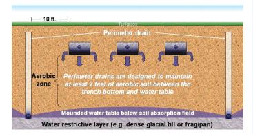
**Figure 5.** Cross-section of a soil absorption field with a perimeter drain installed around the trenches. Indiana requires at least 10 feet between the soil absorption field trenches and the perimeter drain. The drain is intended to lower seasonally high water tables and maintain the aerobic zone below absorption field trenches.
