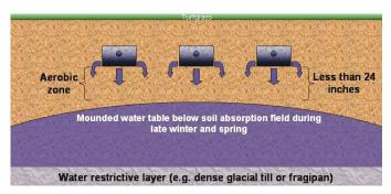
**Figure 3.** In late winter and spring, the mounded water table above the restrictive layer is much higher. Adding wastewater to this high water table can reduce the area of the aerobic zone beneath the soil absorption field trenches to less than 2 feet.
