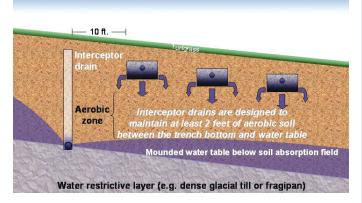
**Figure 7.** Cross-section view of a soil absorption field with an interceptor drain on a sloping site. Interceptor drains are similar to perimeter drains, but are only installed on the upslope sides of soil absorption fields.
