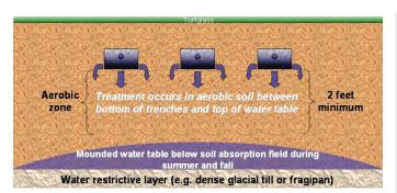
**Figure 2.** Cross-section of a typical septic system soil absorption field during summer and fall, showing a mounded water table above a restrictive layer (such as dense glacial till or fragipan).
