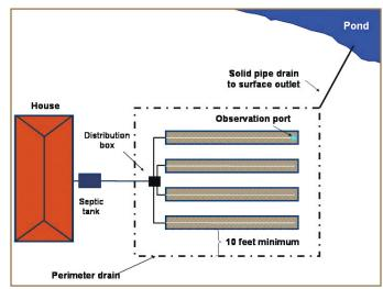
**Figure 6.** A perimeter drain is constructed of perforated polyethylene pipe placed at the bottom of a gravel-filled trench surrounding a septic system soil absorption field. A junction is installed at the lowest elevation of the perimeter drain trench and the drain is connected to a solid pipe to transport water to a nearby ditch, stream, or pond, or to a lower part of the lot.
