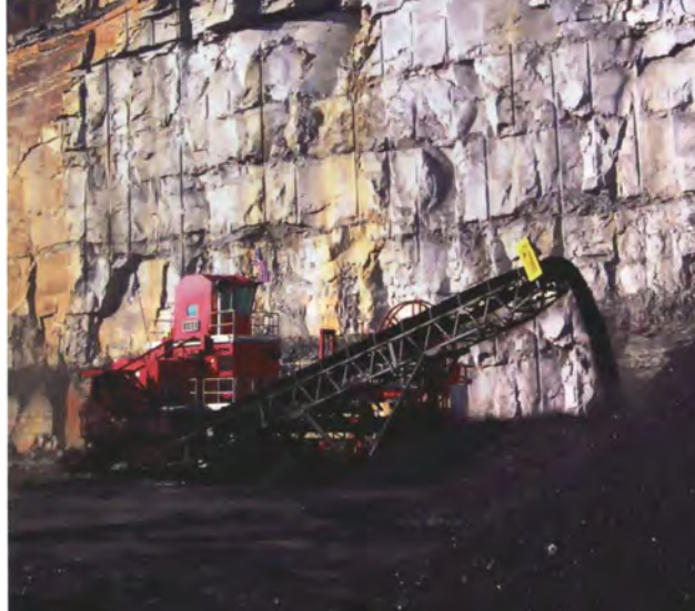
Contour Mining's Powelton highwall miner averages more than 60,000 tons per month. *Coal Age, August 2009
