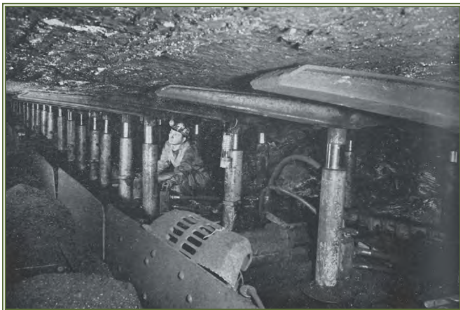
Self-advancing roof support system reduces manpower more than 50% and effectively controls the roof. *Coal Age, December 1961
