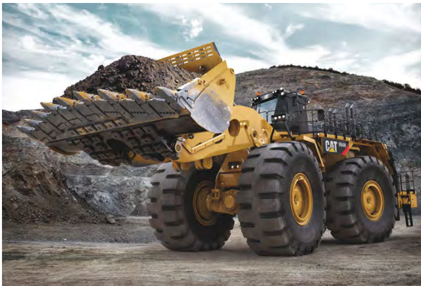
The Cat 994 wheel loader is optimally matched to the 270-ton 793 haul truck.
