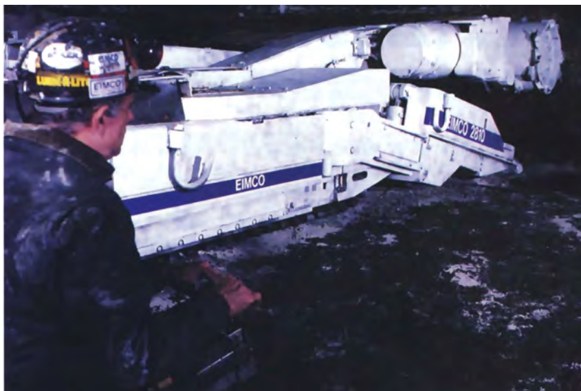
Eimco model 2810 continuous miner is designed for mid-seam mining. *COAL, January 1990
