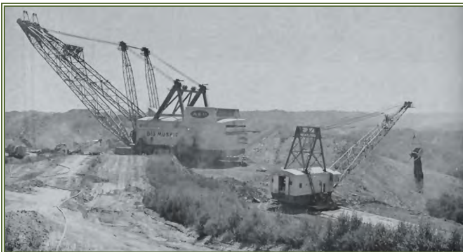
Side-by-side views show a 12-yd dragline (right) leveling working bench for Big Muskie, the giant 220-yd machine. *Coal Age, December 1969
