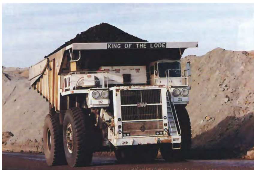
Black Thunder, one of the first Powder River Basin mines to test and adopt Wiseda's 240-ton hauler (shown above), now owns 11 of them. * COAL , July 1993
