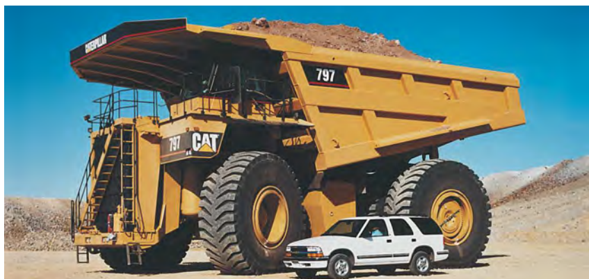
Cat predicts its 360-ton-capacity 797 mining truck will deliver 5% to 10% better fuel cost per ton, as well as 10% to 15% lower overall operating cost per ton. * Coal Age , April 1999
