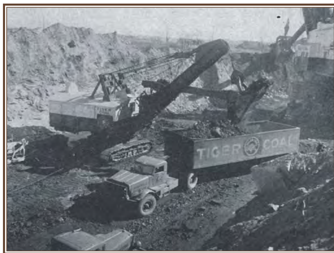
Getting a load of about 75 tons of coal in the Tiger pit. This butane-electric tractor and semi-trailer, rated at 80 tons, has just turned in the space in front of the loading shovel. * Coal Age , August 1939
