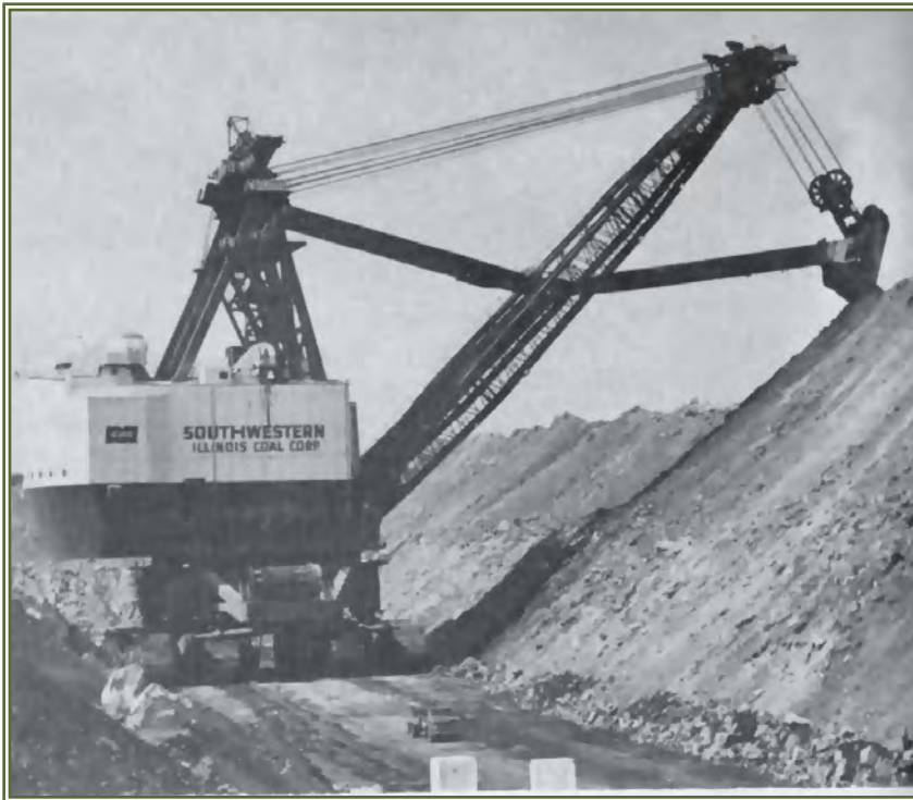
As the Captain stretched to dump its 270-ton load, its size required that the rear of the house swing over the upper seam. The interval between the upper No. 6 and lower No. 5 seam is about 25 ft. *Coal Age, December 1967
