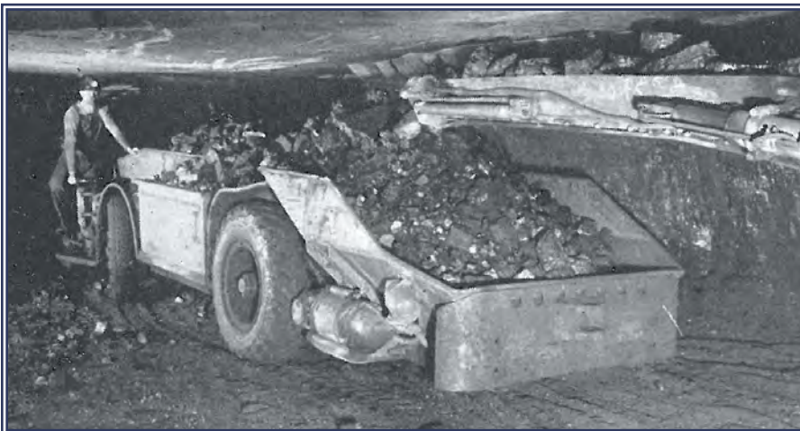
Shuttle car getting a load of more than 6 tons of coal. * Coal Age , February 1941
