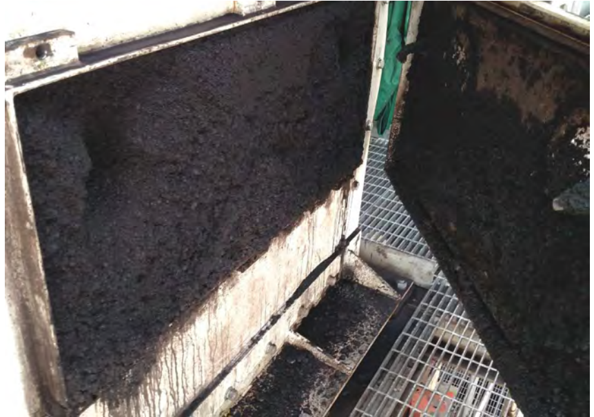
The downtime associated with coal chute blockages can cost thousands of dollars per hour in lost production.
