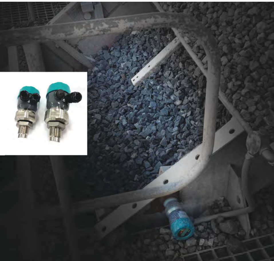
Microwaves can also be used to monitor material flow. The sender units can be seen in the inset.
