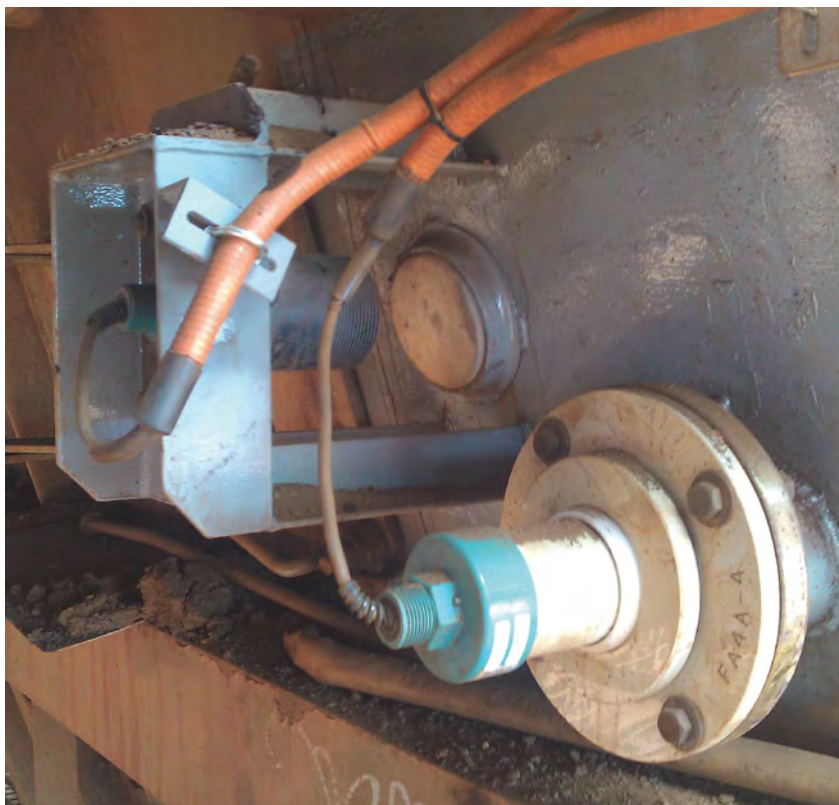
An acoustic switch can be mounted to a chute to monitor material levels.
