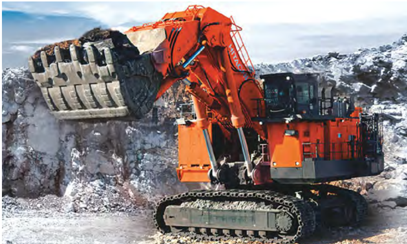
Available in backhoe and front-shovel configurations, the EX5600-6 hydraulic excavator is now offered in diesel- and electric-powered configurations. It comes equipped with Hitachi's Global e-Service remote machine management system, which allows managers to access the machine remotely using the internet.
