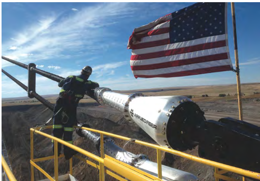
The terminating end of a pendant, which was made from synthetic rope, can be seen on a dragline in Wyoming.
