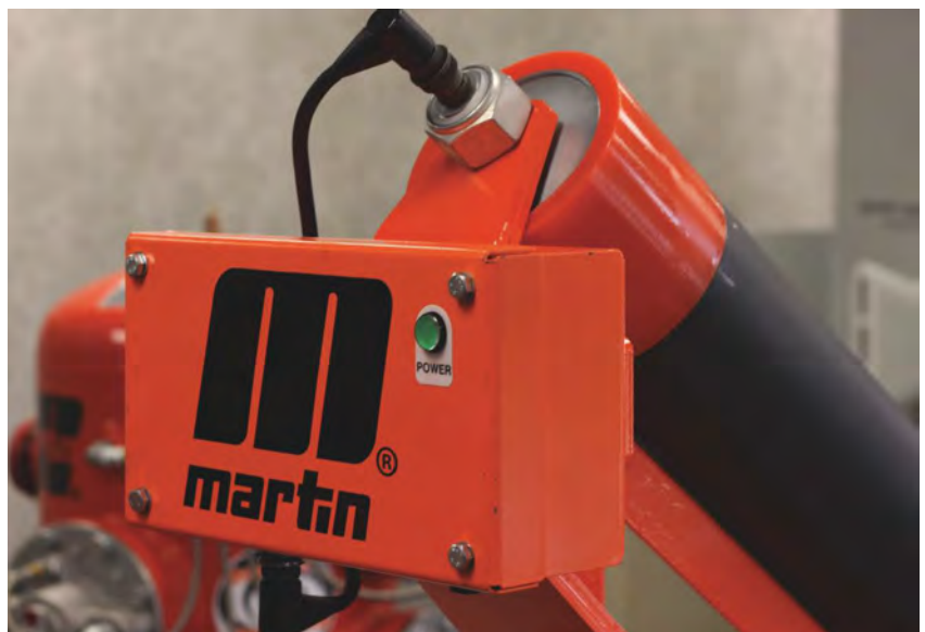
The Roll Gen System acts as a self-contained mini power station.
