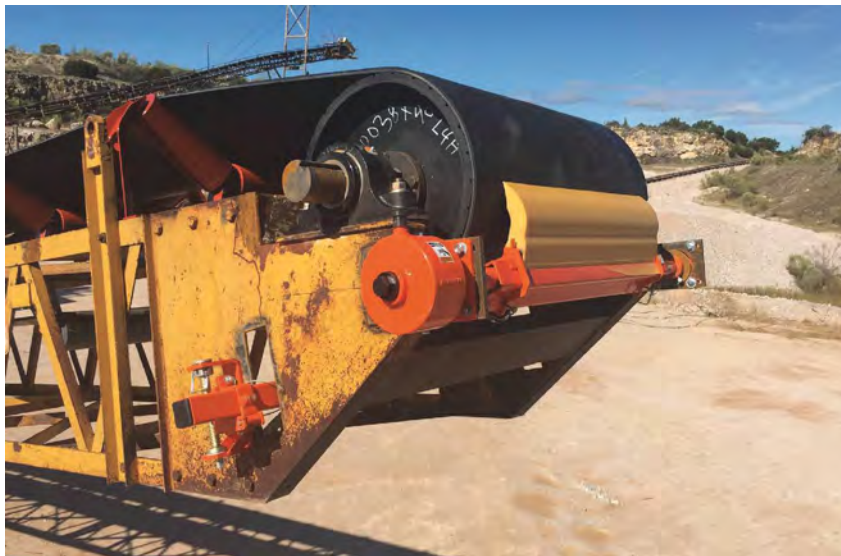
The QB1 Cleaner HD has an alignment system for precise installation.
