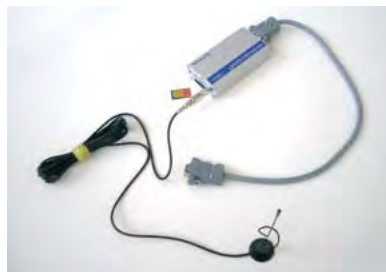
Accessorio per collegamento remoto al PLC della macchina Accessory for remote connection to machine PLC
