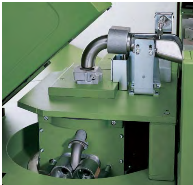
◀ Convogliamento nastro e coiler Sliver threading and coiler
