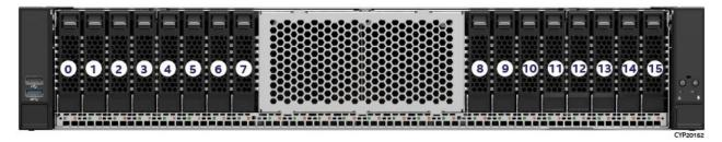
Figure 71. 16 x 2.5" Front Bay Drive Configuration – M50FCP2UR208 with accessory options
