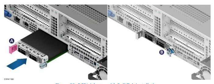
Figure 58. OCP\* Adapter with Pull Tab Installation
