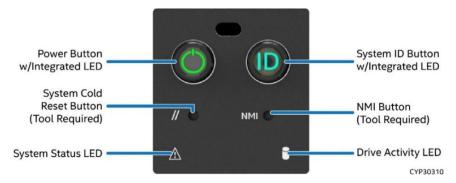
**Figure 93. Front Control Panel Features**
