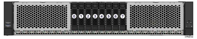
Figure 70. 8 x 2.5" Front Bay Drive Configuration – M50FCP2UR208
