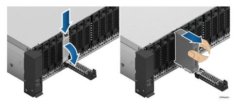
Figure 61. 7-mm Drive Removal from 2.5" Drive Bay
