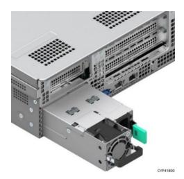
Figure 29. 2100 W Power Supply Module Partially Out of Chassis
