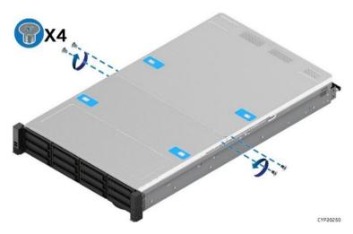
Figure 23. Top System Cover Panels Shipping Screws
