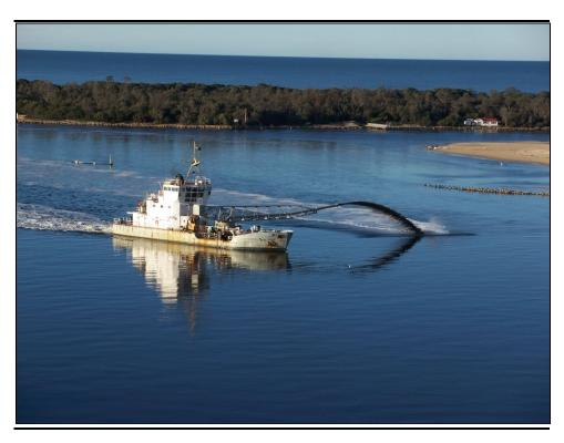
*Figure.4 Typical TSHD (material stored on board for disposal at appropriate location)*
