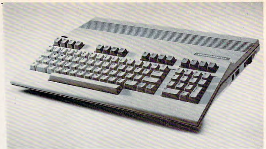
Commodore 128 Personal Computer: a unique three-in-one machine, containing a 64K Commodore 64, a 128K Commodore 64, and a Z80 CP/M computer.
