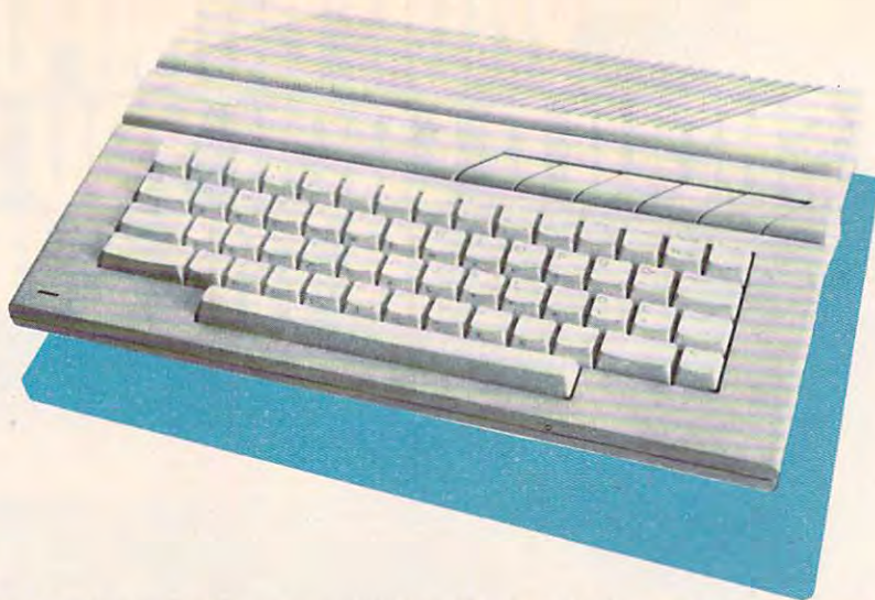
Atari 65XE: basically a remodeled 800XL for $99. Note the resemblance to the ST series. The 130XE, 65XEM, and 65XEP are similarly styled.
