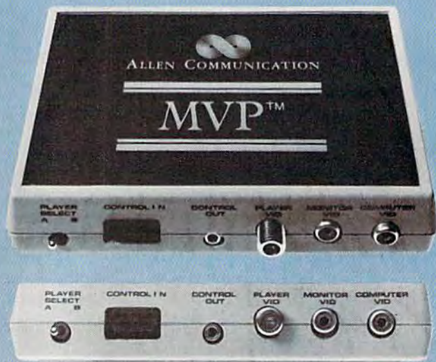
The MVP interface lets Commodore 64 and 128 users connect their systems to a variety of videodisc players.
