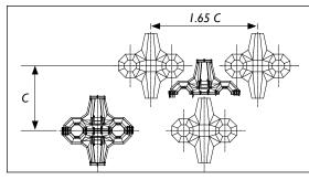
Plan layout of casting arrangement
