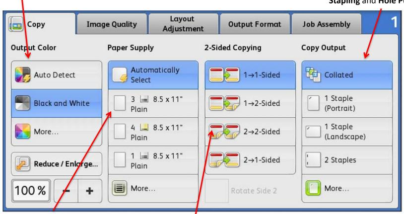
Paper Supply: This is where you can choose an individual tray. When it is on Auto Select the machine will determine which tray to pull from the originals size.
