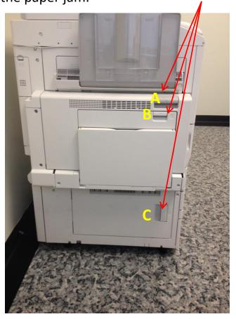
Anything green colored is the paper path and where the jam would occur. Make sure to open or twist the green knobs before pulling the paper out.
