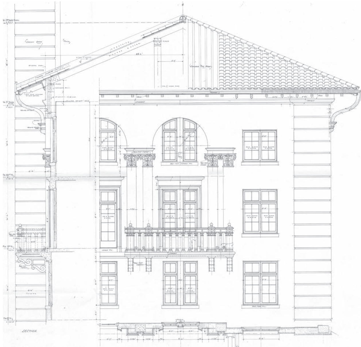
Side Elevation and Section Detail, Wing
