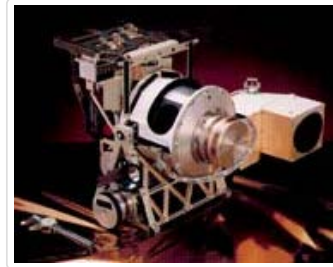
This SeaWiFS (Sea-viewing Wide Field-of-view Sensor) is an ocean color sensor.
