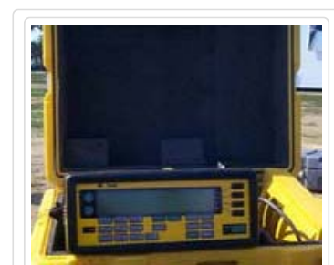
Portable GPS unit utilized in surveying.
