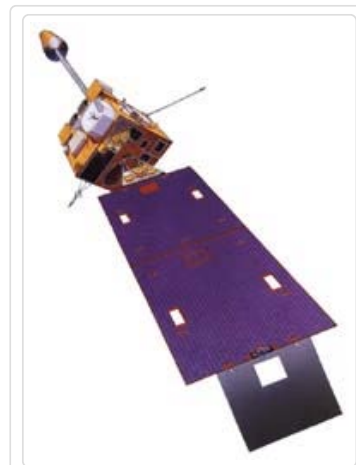
Artist's rendition of GOES I/M, geostationary satellites whose mission includes data collection and broadcasting, and environmental sensing. (Image: NASA/Goddard Space Flight Center)
