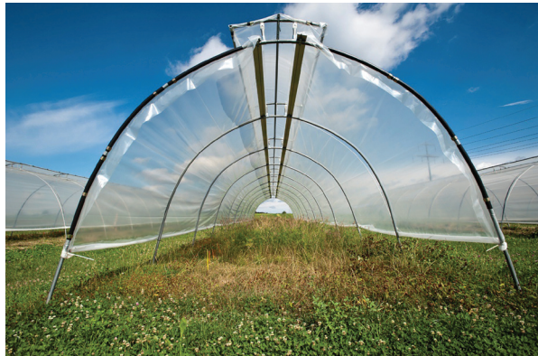
Photo: Rain out shelter used to simulate drought stress by excluding all the rain during a period of 18 weeks.
