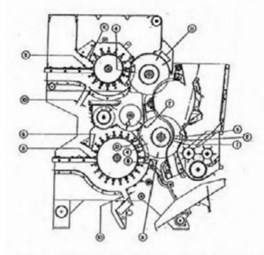
Figure 8. Hardwicke-Etter Super Regal 200 and 252 Dual Saw Gin. Important noted settings and adjustments are given in the text.
