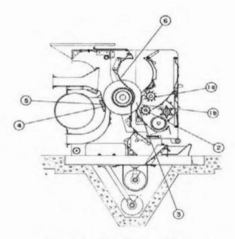
Figure 16. Moss-Gordin 16-in. Saw Air-blast Gin.
