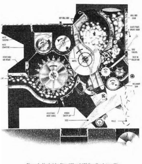
Figure 6. Hardwicke-Etter 100 and 120 Saw Brush-type Gin.
