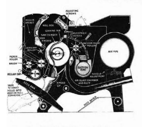
Figure 5. Hardwicke-Etter CXX 120 Saw Air-blast Gin.
