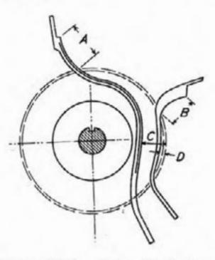
Figure 27. Critical saw-rib dimensions (A, B, C, and D) that vary with manufacturer's make and model.
