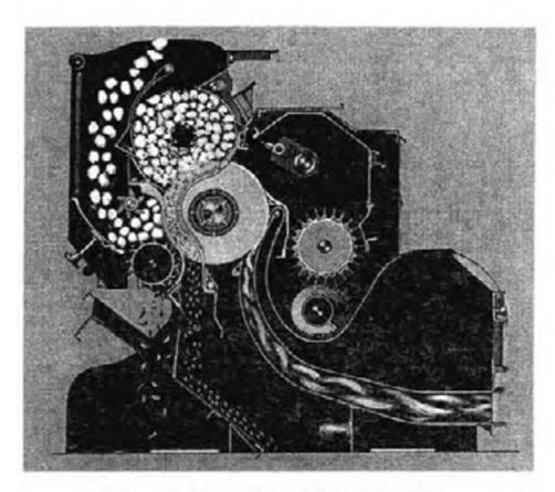
Figure 10. Murray 90 Saw Safety Air-blast Gin.
