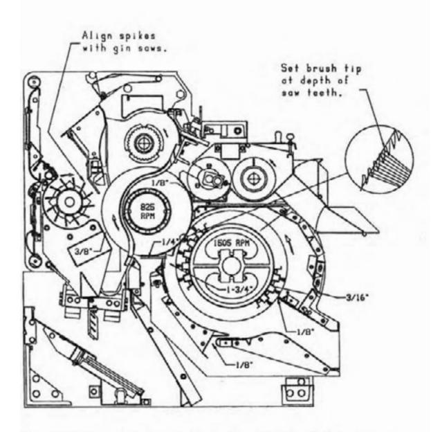
Figure 24. Settings and adjustments for Lummus Imperial II 108 and 158 Saw Gins.
