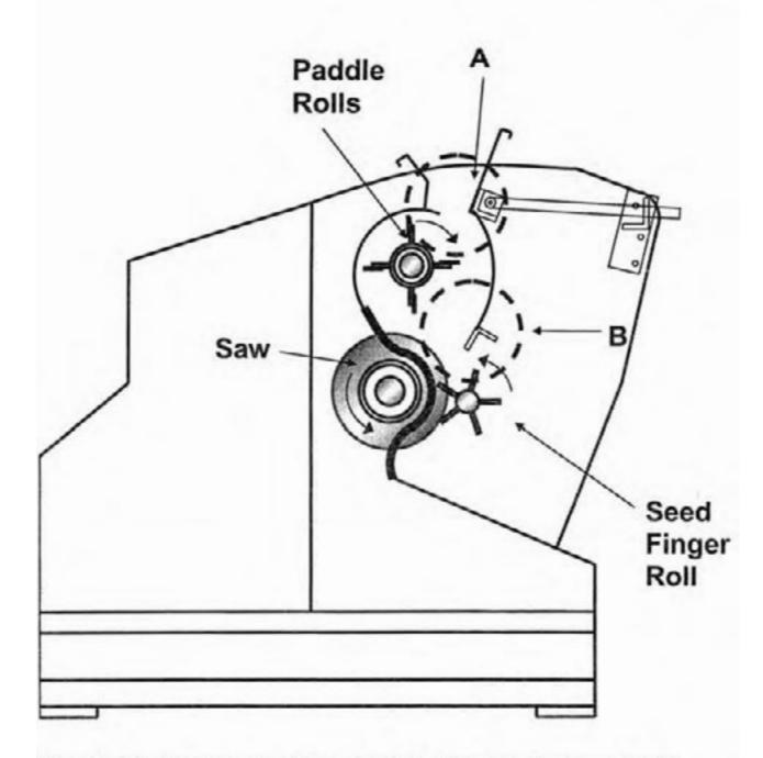
Figure 30. Schematic cross section of Powered Paddle Roll Gin Stand. Circled areas A and B required major changes from the conventional layout.
