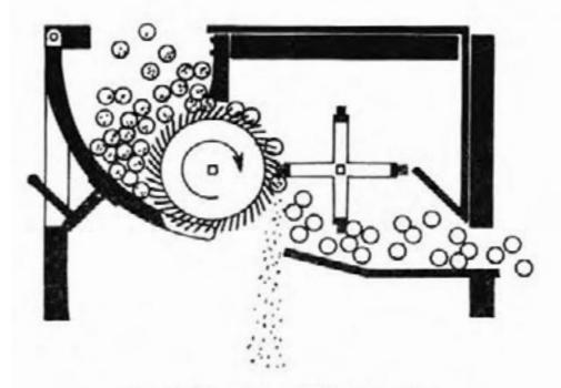
Figure 3. Cross-section of Whitney-type Gin.
