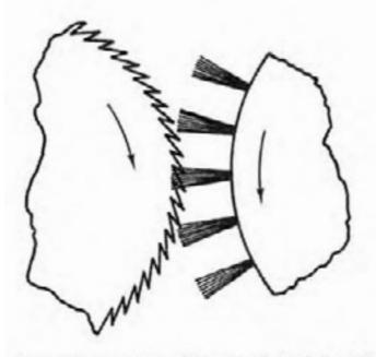
Figure 29. For proper doffing, the gin brush should be set to mesh with the depth of the sawteeth.
