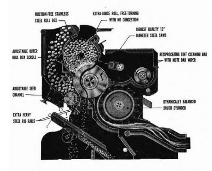
Figure 11. Murray 120 Saw Safety Brush-type Gin.
