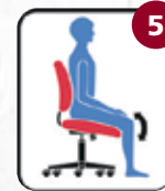
5 Seat Angle Adjustment Allows seat to tilt forward changing the angle of your thighs
