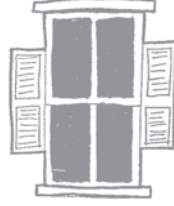
Inappropriate: shutters are too small and shutters do not cover entire window when closed
