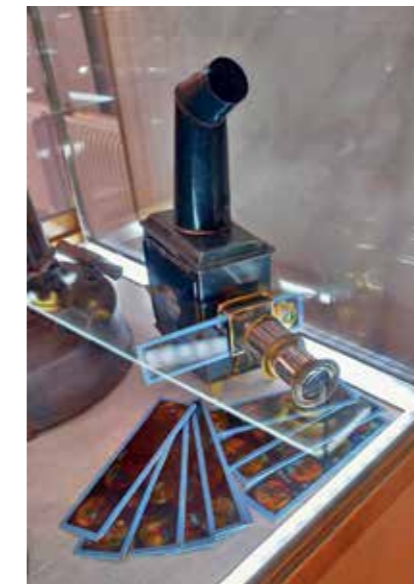
KEROSENE SLIDE PROJECTOR. ERNST PLANCK, LATE 19TH CENTURY INSIDE IS A MINIATURE WICK KEROSENE LAMP 8 CM HIGH. AT THE TOP: CHIMNEY
