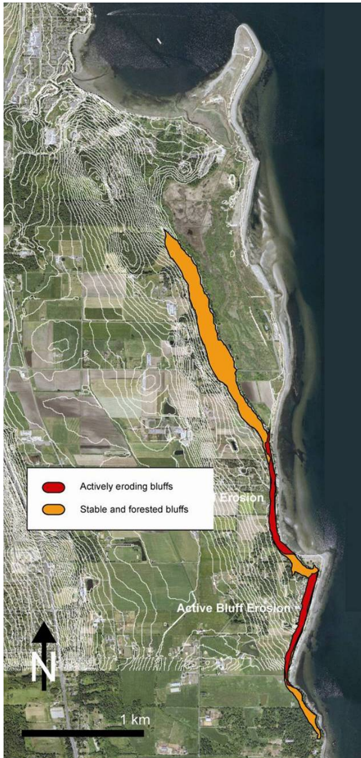
Figure 12. Location of bluff ecosystems in Cordova Shore. The red polygons show the location of actively eroding bluffs at Cowichan Head. Note that the bluff transitions to more gentle upland near the northwest corner of the Tsawout Wetland.
