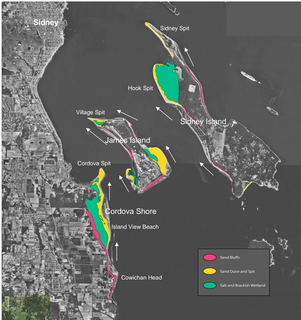
Figure 3. Sand bluffs, dunes, spits, and coastal wetlands in the Cordova Shore-James Island-Sidney Island area of southern Strait of Georgia. Feeder bluffs are shown in red, coastal sand ecosystems are shown in yellow, and coastal wetlands are shown in green. The prevailing direction of sediment transport is shown with white arrows (from the south and southeast).
