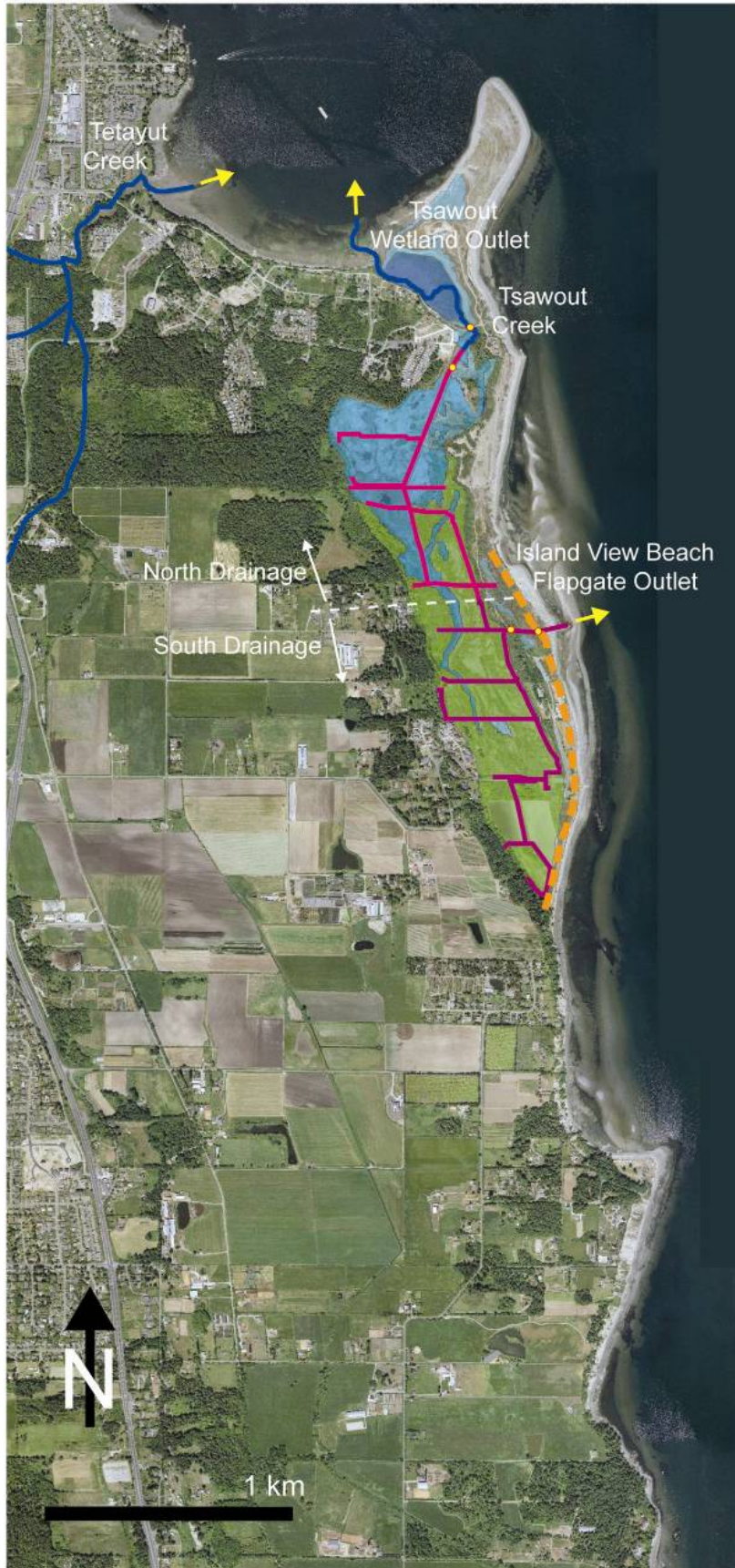
Figure 14. Drainage system of the Cordova Shore. It includes natural channels (dark blue), and two manmade drainage systems: the North Drainage (pink) which includes the salt and brackish marshes and drains to Saanichton Lagoon through Tsawout Creek; and the South Drainage (purple) which drains Island View Beach and the farmlands to the south and discharges through a flapgate. The drainage systems are connected. The shoreline protection dike is shown with a dashed orange line.
