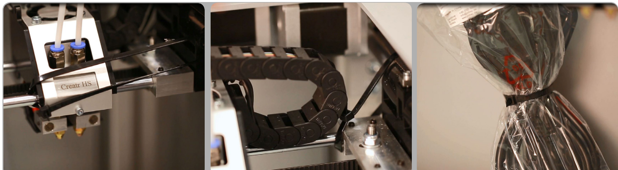
STEP 4: Cut the tie wraps at the front and back of the carriage and in the back of the printer
