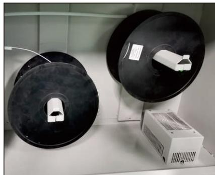
Filament dry room have 2 temperature options to set. (45 degree /65 degree.)
