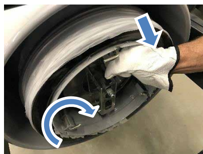
9- Pull and rotate the retaining pins and insert them into their seats.
