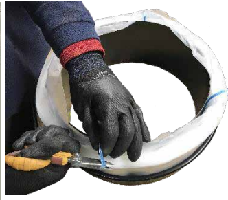
5- Cut and remove the LONGOPAC® closing bands.
