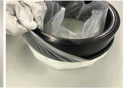
7- Pull the outer part of the bag to create the new one.
