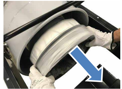
3- Remove the LONGOPAC® container and any waste.
