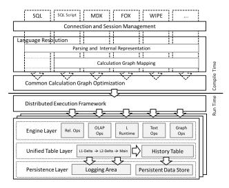
Figure 2: Overview of the HANA database layered architecture
