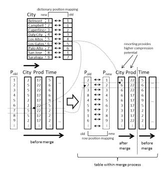
Figure 8: Delta-to-main merge with reordering
