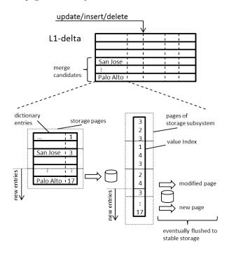
Figure 6: Details of the L1-to-L2-delta merge
