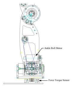
Fig. 5 Ankle joint design
