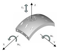
Fig. 4 Hip yaw actuator output frame
