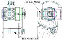
Fig. 3 Hip-roll and pitch joint design
