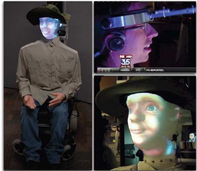
Figure 2: Left : Current PVA prototype, with a real human agent and appearance. Top Right : Real human appearance obtained from a head-worn camera. Bottom Right : Real human agent but synthetic appearance from the teacher training system.
