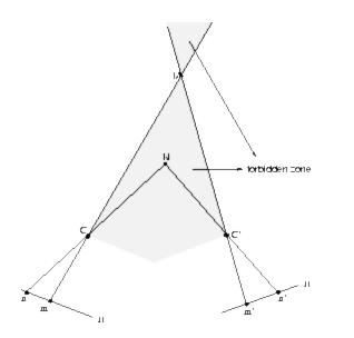
The ordering constraint fails if a given 3-D point (*N* here) falls onto the forbidden zone of another 3-D point (*M*). In the left image (\$\Pi\$), *m* is to the right of *n*, but in the right image (\$\Pi\$), this ordering is reversed.
