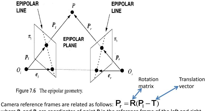
where  $\mathbf{P}_{r}$  and  $\mathbf{P}_{l}$  are coordinates of point  $\mathbf{P}$  in the reference frame of the left and right cameras. The image of  $\mathbf{P}$  in the two image planes has coordinates  $\mathbf{p}_{l}$  and  $\mathbf{p}_{r}$ .
