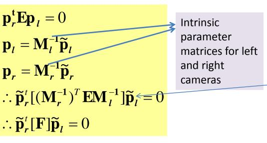
The essential matrix E gives the relationship between the corresponding points measured in camera coordinates. The fundamental matrix F gives the relationship between the corresponding points measured in homogeneous coordinates with the x and y components measured in the pixel coordinate system. F also has rank 2.
