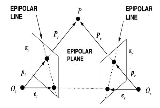
Figure 7.6 The epipolar geometry.
