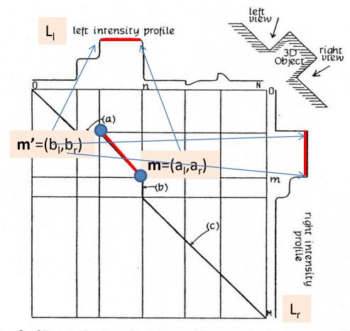
Fig. 3. 2D search plane for intra-scanline search. Intensity profiles are shown along each axis. The horizontal axis corresponds to the left scanline and the vertical one corresponds to the right scanline. Vertical and horizontal lines are the edge positions, and path selection is done at their intersections.
