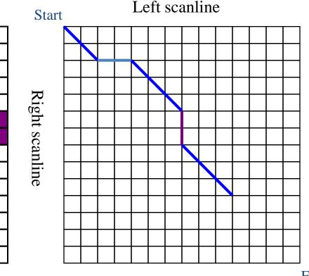
Dynamic programming yields the optimal path through grid. This is the best set of matches that satisfy the ordering constraint
