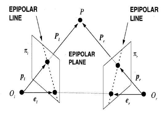
Figure 7.6 The epipolar geometry.
