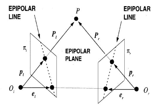
Figure 7.6 The epipolar geometry.
