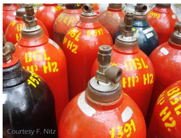
Figure 12: Certain gas cylinders were cleaned with carbon tetrachloride (CTC), which is an ODS
