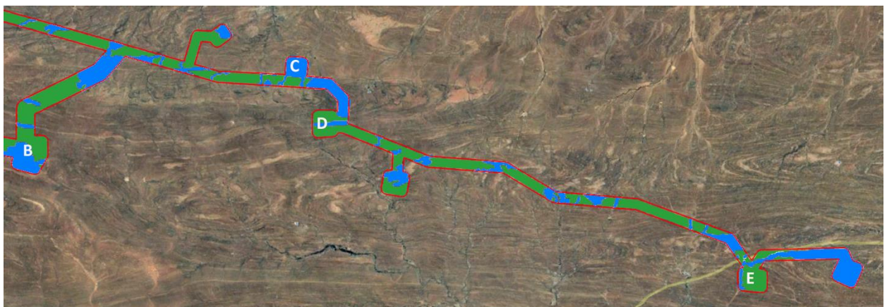
Figure 21: Sensitivity map of the Kwagga OTP route Segment B – E. Blue indicates a moderate sensitivity and green a low sensitivity.
