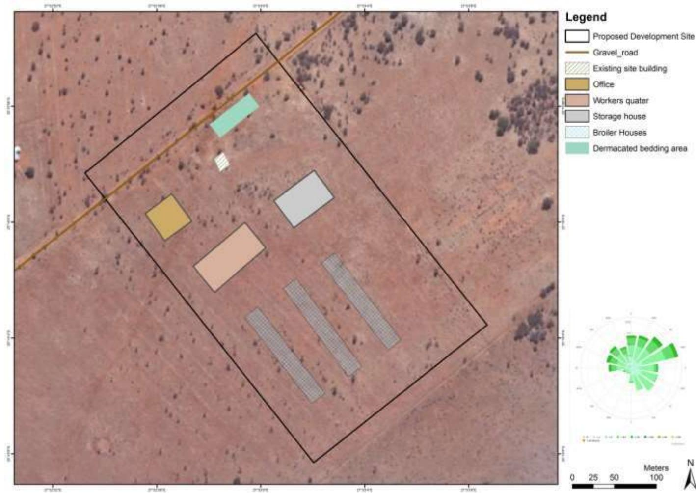
Figure 3: Site layout of the proposed development site (as supplied by the Project Proponent)
