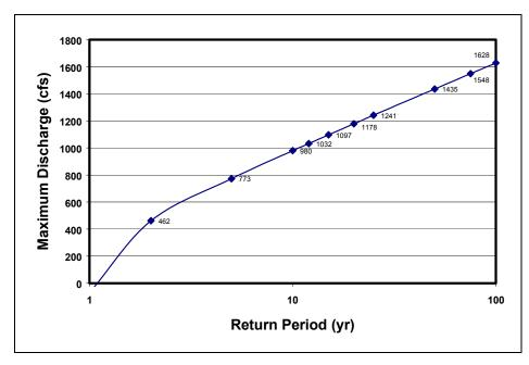
Figure 5. Flood Frequency Curve for Big Chico Creek during Spawning Period 1 (February).
