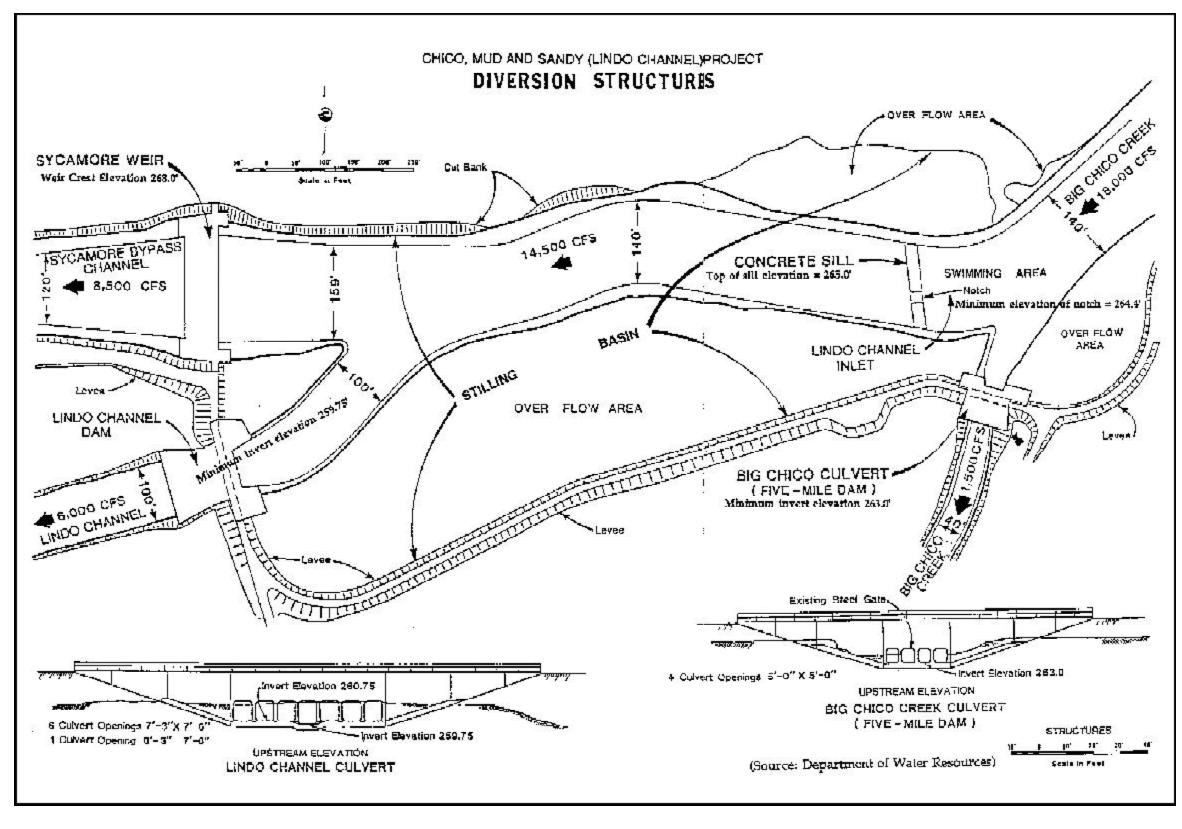
Figure 1. Diversion Structures
