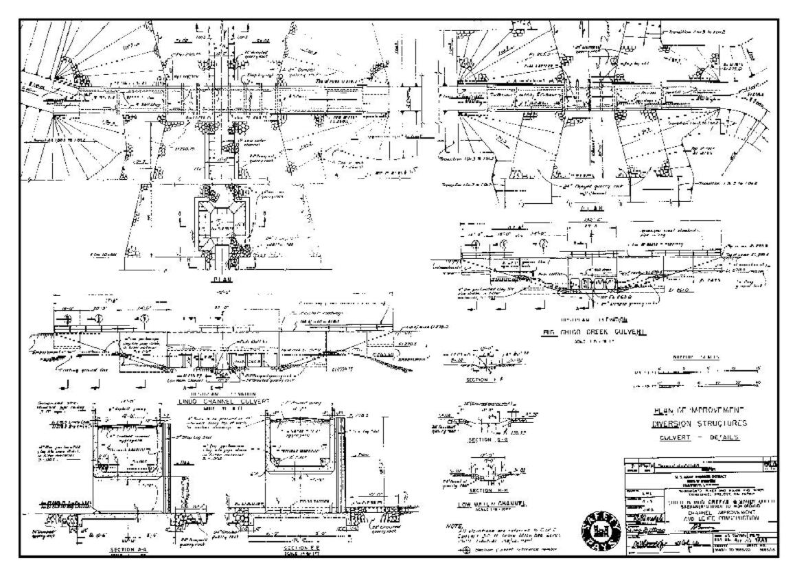
Figure 3. Diversion Structures Improvement Plan - Culvert Details.
