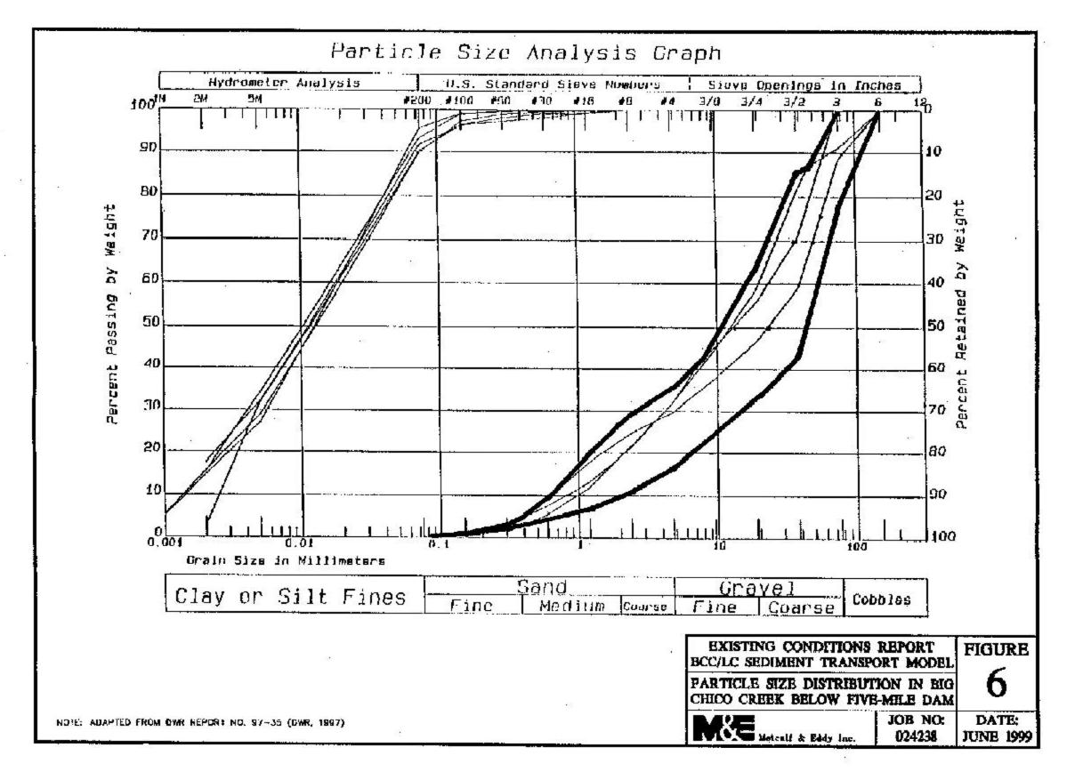
Figure 8. Particle size distribution in Big Chico Creek below Five-Mile Dam. Source: Medcalf & Eddy Inc. (June 1999)
