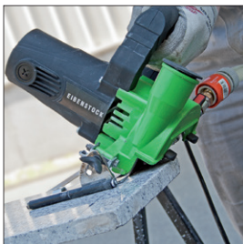
Stepless mitre adjustments up to 45° – without tools
