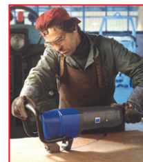
CS-3400 cuts up to 3/8" thick steel.
